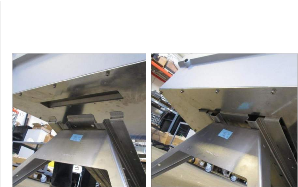
STEP B – ALIGN MOUNTING TAB WITH INVERTER SLOT
